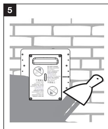
Make sure that the thickness of the plaster is flush with the inlet (about 1 cm) all around the inlet (figure 6).
