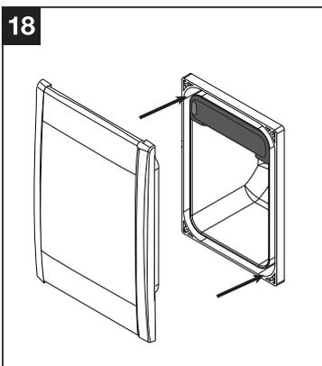
Simply insert the door into the appropriate slot (figure 18).
