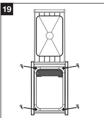
Then, open the door and insert the four screws in the corners (figure 19) to hold the piece in place. Adjust the 4 screws so that the door closes properly.
