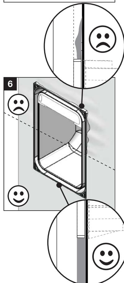
Use as a template to cut the opening in the brick wall.
